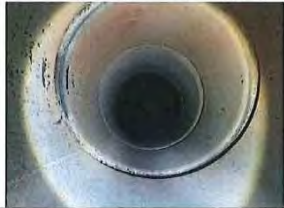
Burner refractory / flame tube joint
